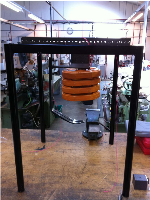
Figure 5. Prosthesis drop test rig.
